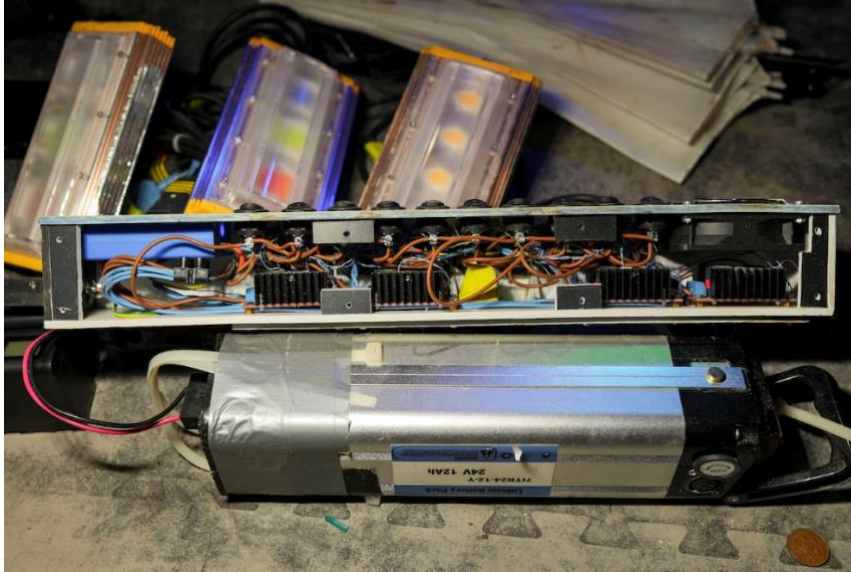
Battery and controller. daz disley, 2023.
